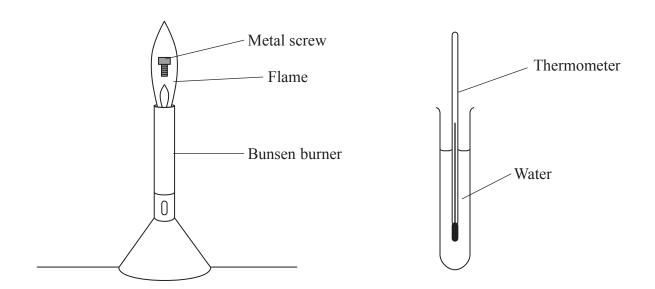
The thermal energy lost by the screw raises the temperature of the water so that energy lost by screw in cooling down = energy gained by water in heating up For both the screw and the water, energy transferred  $\Delta E$  is given by
