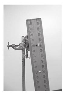
The rule is rotated through a small angle and released. It then oscillates about the pin as a pendulum with a time period T.
